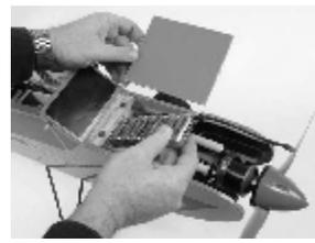
12. Installation of battery and front hatch. Note the two circles in front of windshield; those are strong hatch magnets to hold hatch closed.
