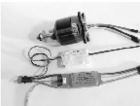
12. Solder all connectors for motor, speed control, battery, and BEC. (Note: use instructions supplied with each item. Look how this particular BEC is wired into speed control at battery connector.)
