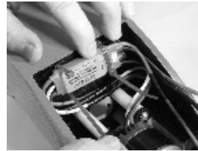
17. Install speed control on front-bottom of firewall (shown upside down)
