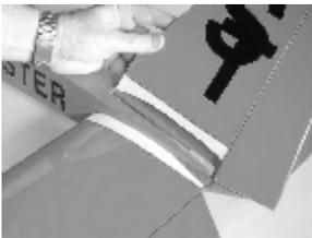
10. Install vertical stabilizer into slot and check for 90° angle to horizontal.
