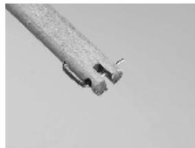
15. Each pin will point toward tail of aircraft. Use small rubber bands or tape to safety into position.
