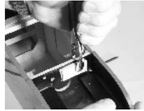
4. Use channel-lock pliers to press blind nuts into position (note: drilled hole should be slightly smaller than shaft of blind nut for tight fit).
