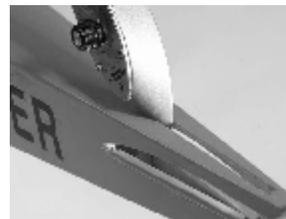
1. Cut covering and iron edges into slot.
