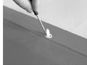
4. Install aileron horns so that pushrod is 90° to hinge line.
