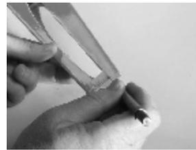
2. Cut and remove the elevator spacer at rear of fuselage.
