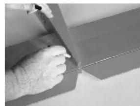
6. Mark position of tail by drawing along all four corners. (Note: be careful not to move tail during this step, as these lines will be useful when glues tail to fuselage)
