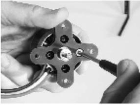
10. Install engine mount plate with supplied flat-head screws.
