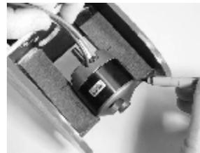
6. Rest motor on mounts. Mark approximately 1/4" wider than engine on both sides with pen.
