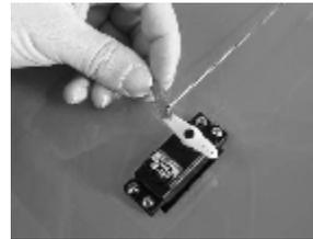
5. Install plastic pushrod connectors on servo end. Repeat for other side.
