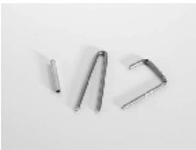
6. Locate these parts.(or fabricate these parts from 1/16" music wire and brass tubing.)
