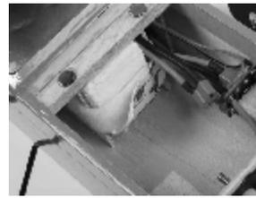
13. Battery is held in by Velcro strap. Cut two 1 1/2" strips of Velcro "hook" and stick/CA to each side of box. Cut 7" Velcro "loop" for strap.
