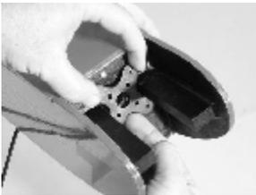
1. Hold the motor mount back plate in place (note: rotate mount till it looks like an "x") and mark the screw locations with "ultra-fine sharpie" marker.
