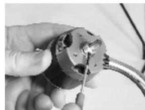
9. Install supplied engine shaft collar and tighten with hex key.
