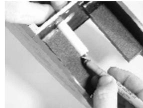
5. Install two 1" spacers with 3" screw into top left engine mount hole. Mark the forward end of the spacers. Repeat on the top right side.
