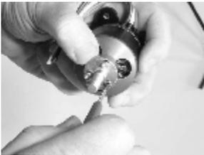
11. Install prop shaft adapter with supplied allen-head screws.
