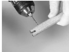
13. Install pin and mark with pencil. Drill 1/16" hole as above for "U-pin" that will lock into wood.
