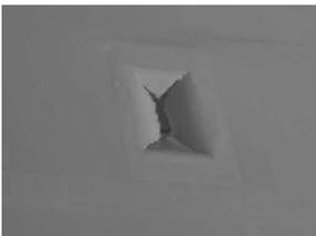
1. Cut holes for aileron servos in an "x" pattern.
