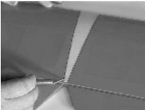
7. Remove covering inside lines. **DO NOT CUT** into wood during this step. Use new blade and cut at angle while pulling covering upward.
