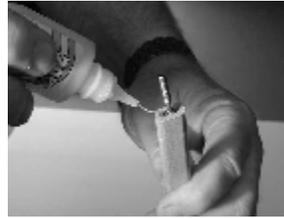
9. Glue flush into top of each strut.
